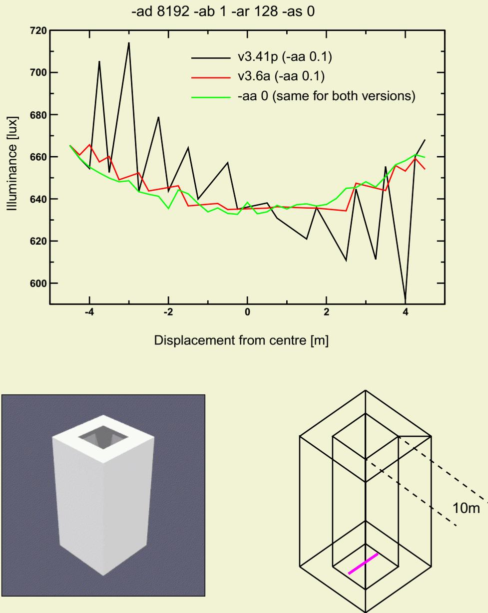
Figure 1. Illuminance profiles with rendering and line drawing of atrium model.
